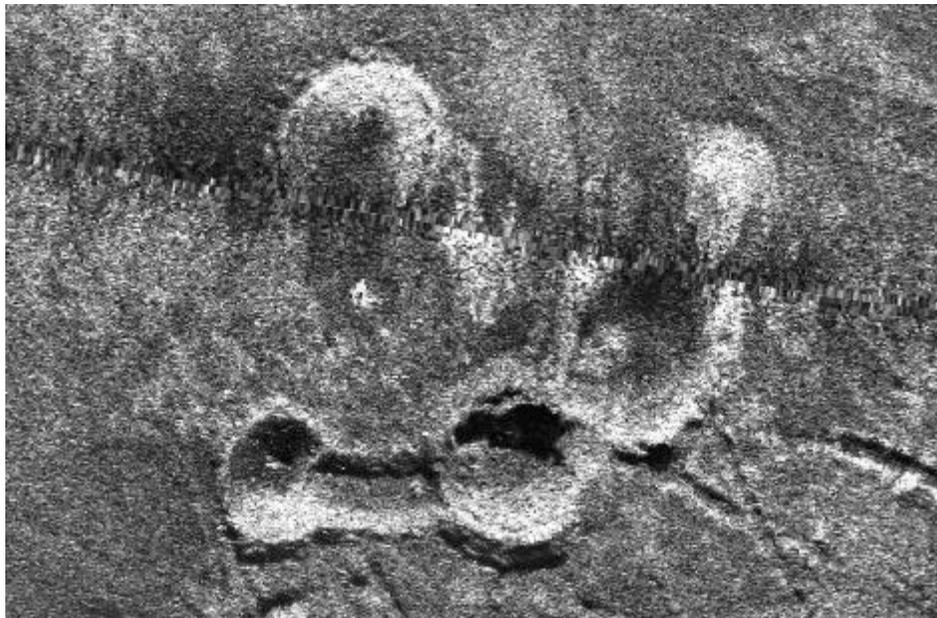
Figure 6a – Conventional Sidescan Image of Oil Rig Scours
