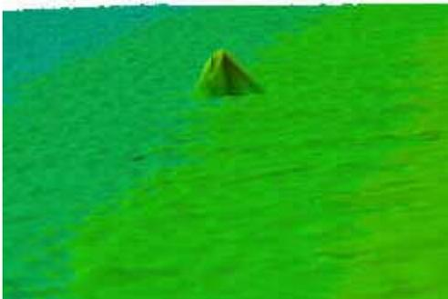
Figure 5a – 3D Manta Mine Shape illuminated by Reson 8125
